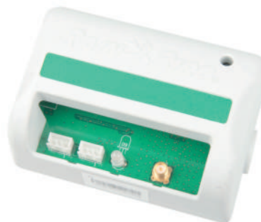
Módulo Radio Master (MRM) IQ TBOS
